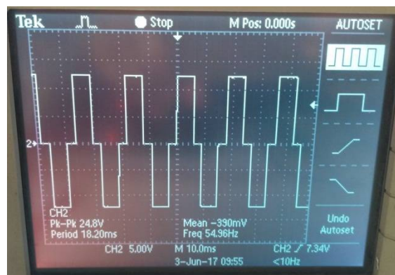
Figure 7 (a) Hardware model output (line-line) voltage of Inverter
